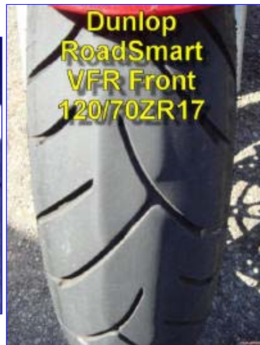
Single compound front.
